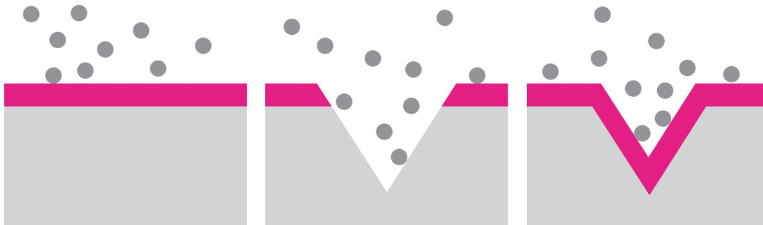
Understanding this process is important for, among other things, the use of stainless steel in low-oxygen or oxygen-free environments; here there can be no subsequent passivation of the surface and the material is exposed to the aggressive influences.
